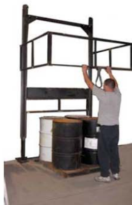
When "corral" is raised, ledge gates swing closed. Worker has access to load. Fall potential is eliminated.
