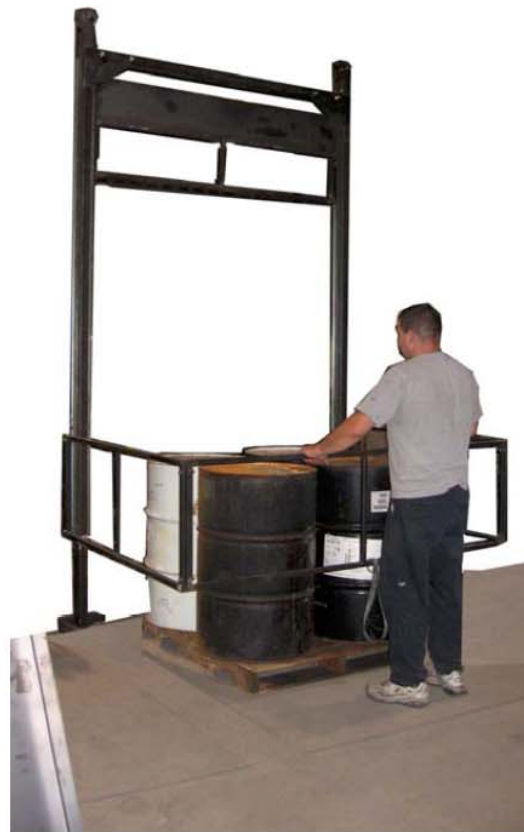
When "corral" is lowered, ledge gates swing open. Worker is blocked from staging area.
